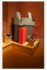
**IBM** - This is an IBM COMPUTER made in the seventies that worked with perforated card. The memory was contained in two disks, one fixed and one mobile.
